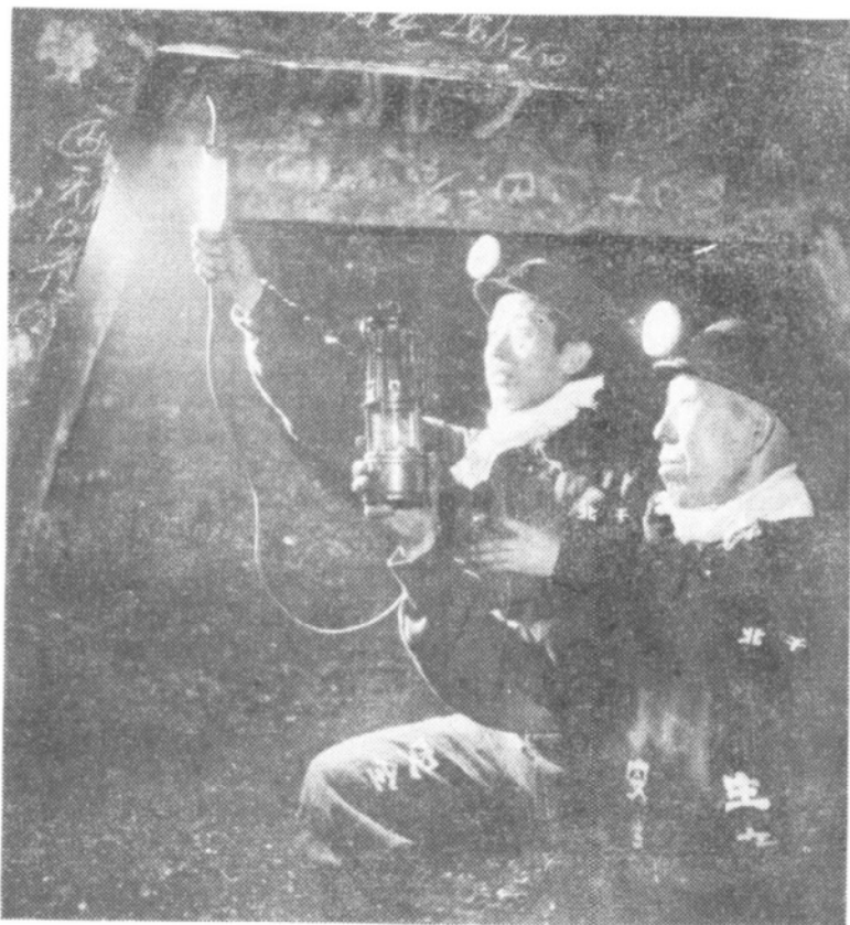
Checking for gas in the shaft.
