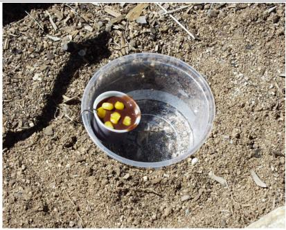
Once the Reifschneider Rain Shield is removed, the wire loop allows the dung cup to be swung out of the way, for easy - and clean - retrival of specimens.
