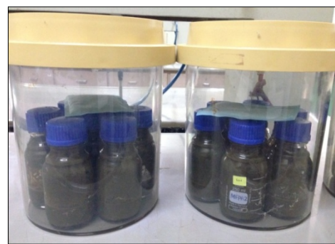
Fermentation Proper: 10 g base material incubated for 14 days in an anaerobic jar
