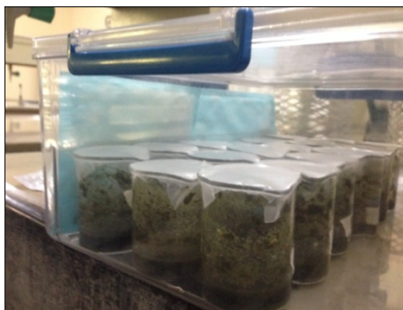
Rhizoclonium riparium powder soaked in water (1:9, seaweed: seawater) and enzyme for 2 weeks
