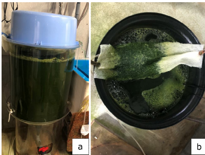
Figure 6. Two types of rotifer rearing tank: (a) Cylindrical glass tank (100 L); (b) Plastic bucket (50
