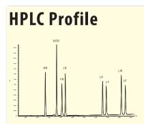
**FIGURE:** Microcystins/nodularin were separated by HPLC on a Waters Sunfire<sup>™</sup> (18 column (2.1 mm ID x 150 mm long; 5 µm particle size) maintained at 40 °C. Mobile phase was Milli-Q water (A) and acetonitrile (B) both containing 0.05% TFA. Components were eluted using a linear gradient from 15% to 65% B over 25 minutes at a flow of 0.3 ml/min.
