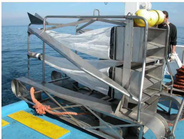
Fig. 2. Epibenthic Sanders sledge dredge equipped with two plankton nets.
