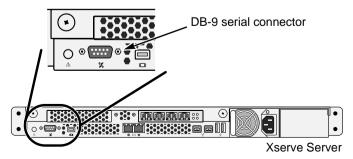
To set up a serial connection with VTrak:
