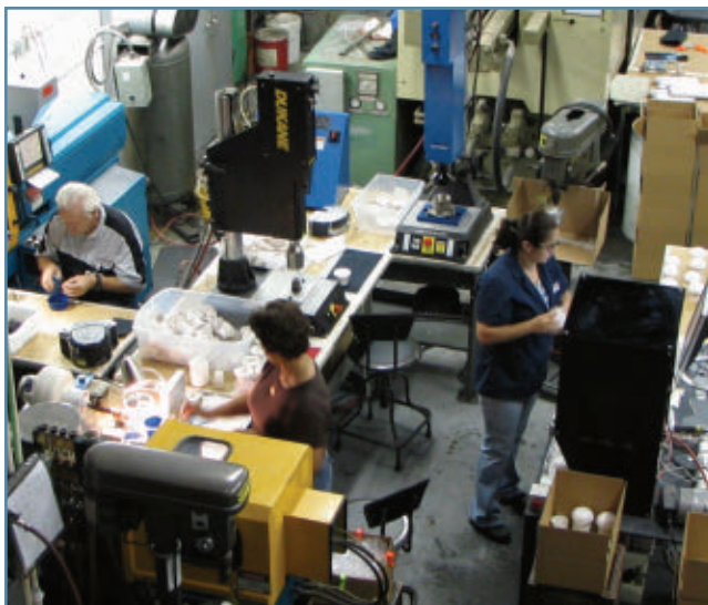
Top These adjustable floats for fishing invented by L.A. Blackwell pushed father and son into the newly forming injection molding industry. Middle Energy-efficient Negri Bossi machines dominate Blackwell Plastics' shop floor. Above This cell creates a finished plumbing device, which requires a seal test. A diaphragm is spinwelded into a housing.
