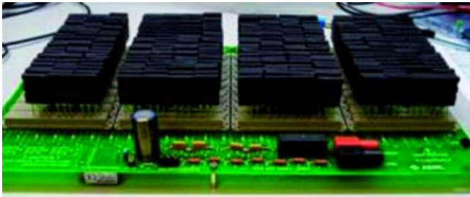
Figure 4: SRB set up for 300 MOSFETs
