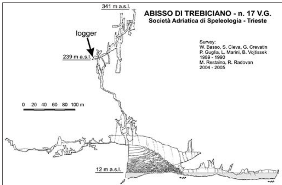
Fig. 1 – Cave survey and instrument location (picture by courtesy of Società Adriatica di Speleologia).
