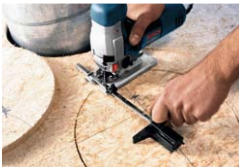
Using the Progressor for Wood and Metal T 345 XF at the construction site, you can cut through not only wood with nails without any problem, but also cut sheet metals, pipes and aluminium profiles.
