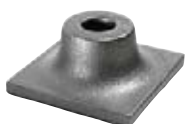
Tamping plate for toolholder 1 618 609 006 or 2 608 690 115 for compressing soil with a working area of 225 cm 2 (1 618 633 104) or 400 cm 2 (1 618 633 105)
