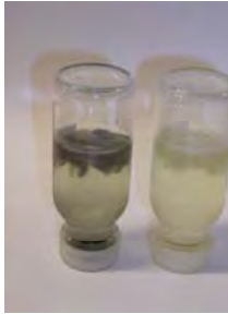
Fig. 4. Sub-cultures of kapok attacked by erosion bacteria in new flasks containing sterilised media, kapok and pine.
