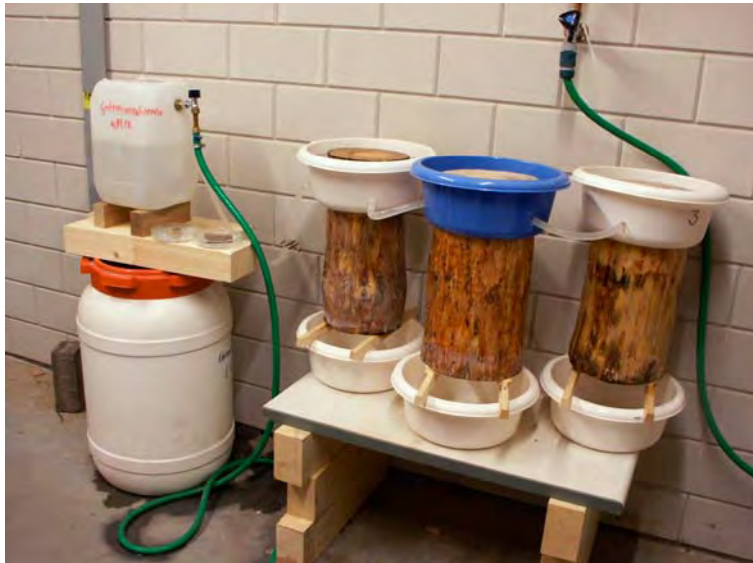
Figure 2. Test set-up experiment water flow trough bark.
