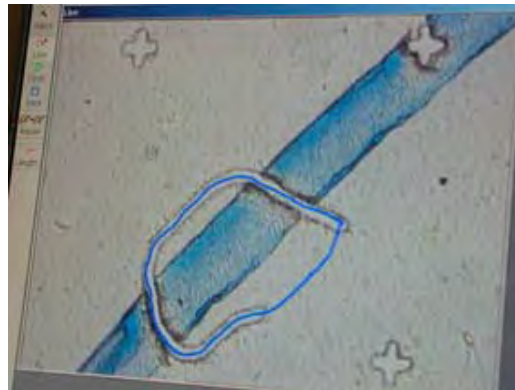
Fig. 12. By using the laser dissection technique it was possible to “cut out” a smaller area on a single kapok fibre for molecular analyses. Photo showing the laser knife in process following the marked line.
