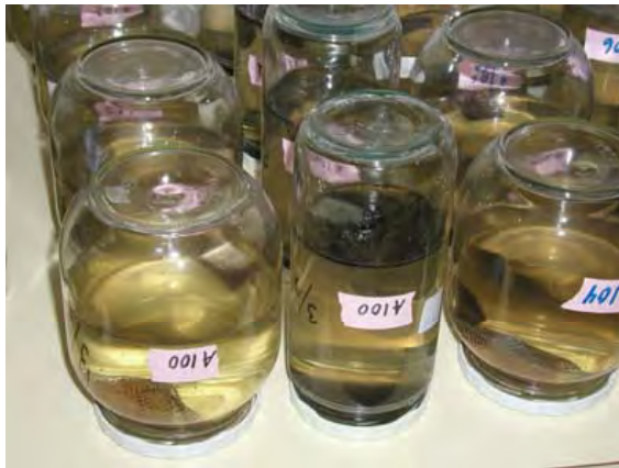
Fig. 1. Original BACPOLES samples incubated in inverted jars with sterilised media, kapok and small pine samples.
