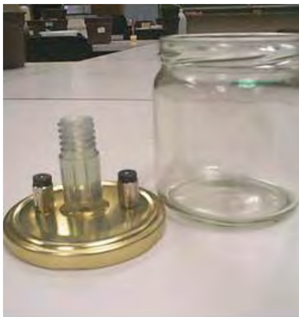
Figure 14. Glass jar and twist off lid equipped with in and out flow valve and septum closed cylinder for water addition
