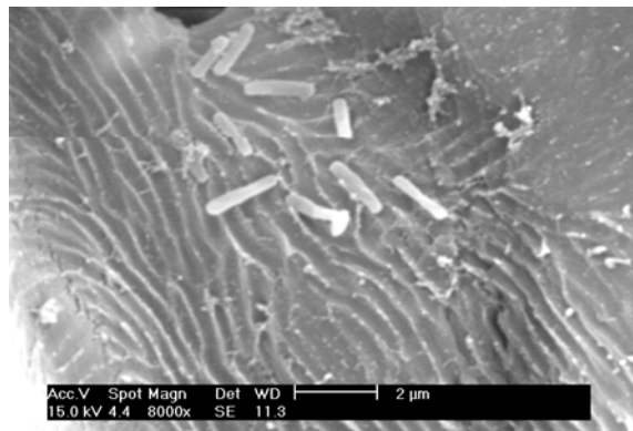
Figs. 7 a,b. Showing active erosion bacteria degrading original BACPOLES foundation pile from site 1, Amsterdam. The rod shaped bacteria are attached to the wood cell wall within their respective troughs orientated along the microfibrils.
