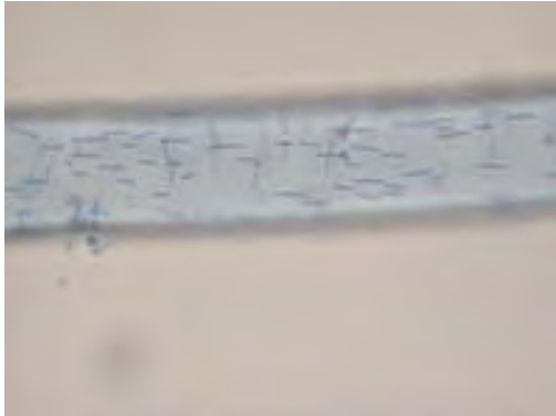
Fig 2. Presence of rod shaped erosion bacteria attached to the cell wall along the microfibrillar orientation of the kapok fibre. X630
