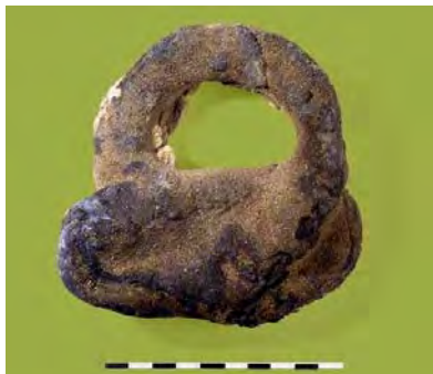
Figure 1: Example of iron object - two iron chain rings - with a scale of FeS-encrusted sand. (De Meern 1)
