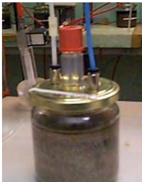
Figure 15. MC filled with sediment and water, and connected to the aeration and GC system
