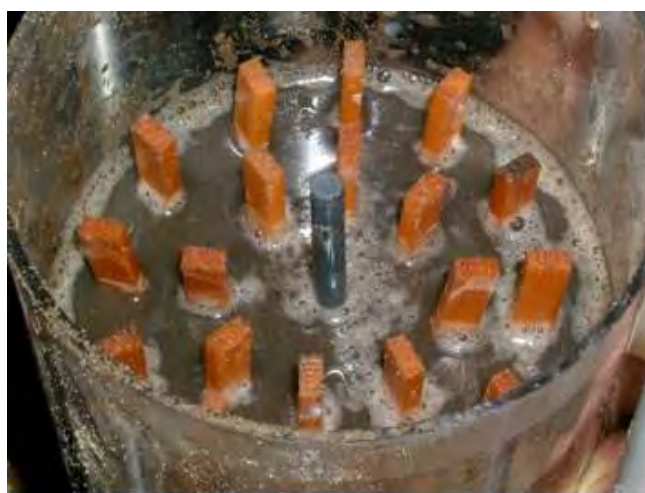
Figure 2. Distribution of the samples of one layer in the Microcosm. (At this stage in the middle of the MC is a plastic stick to keep the space for the attacked wood, added later)
