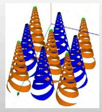
Interspersed conical spiral array
