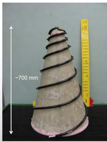
1/3 scale model of SKA-low conical wire spiral antenna
