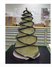
Dual-polarized wire conical spiral prototype
