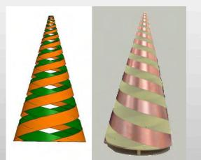
Dual-polarized conical spiral prototype
