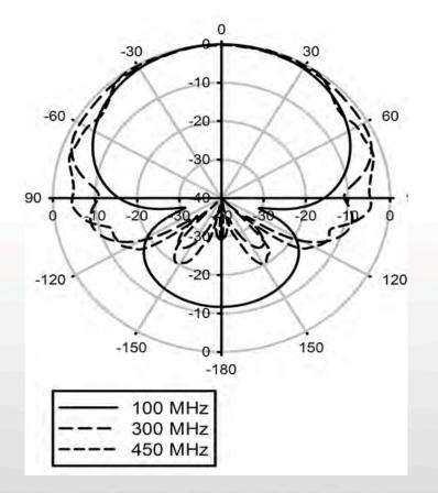
Radiation pattern of wire conical log spiral
