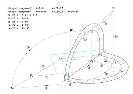
The method is generally applied to the morphologically more complex ashlars – as in the case of the *trompe* of Anet – but requires an accurate calculation of the angles and the shape of the panels since possible errors would accumulate with each phase of cutting.
