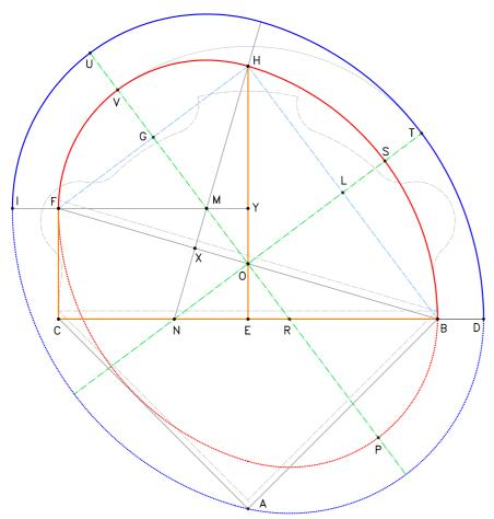
Figure 9 (left). Construction of the internal and external ovals. The two starting point segments are CB, equal to 7.2 feet and EH, equal to 2/3 of CB, 4.8 feet. The triangles EHB and FYH are perfect right-angled triangles 3-4-5. The minor semi-axis of the external oval is congruent to the major semi-axis of the internal oval. The plan of the trompe is shown in by the dotted line in grey, translated by 1/6 foot with respect to the original base CB.
