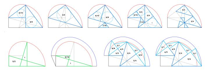
They therefore define the limits of the figure of construction and therefore the shape of the inferior surfaces, the intrados of the rampant vault.<sup>12</sup>
