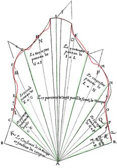
Once a parallelepiped of stone that contains the complete ashlar has been squared, one continues to work along the perpendicular direction to the face of the block, following the projections which are on the face itself.
