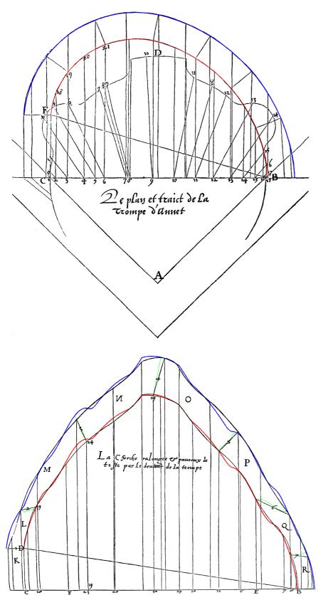
Figure 3 (top left). Delorme, op. cit., f. 96v. Trait used for the construction of the development boards of the trompe of Anet. The ovals obtained by means of the construction presented in the article are highlighted to allow comparison. In the Delorme treatise all diagrams are to the same scale.
