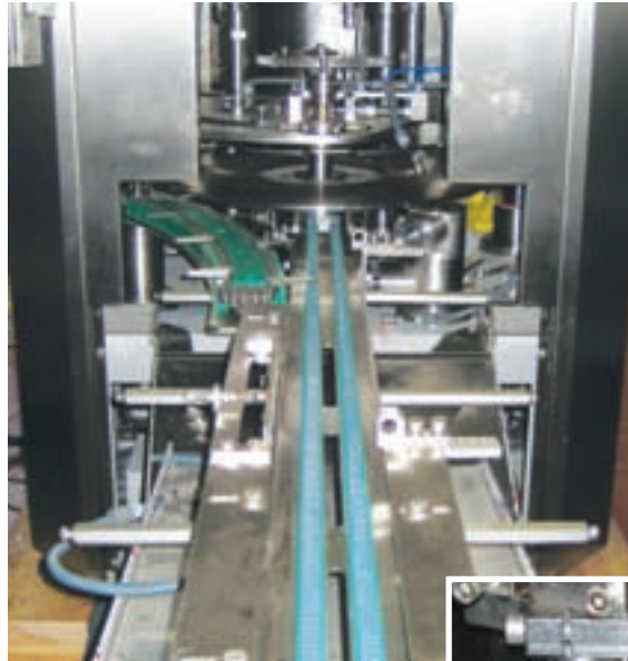
MCG'S R-110 seamer is equipped with a tooling to seam delicatessen fish and shellfish products into tinplate round can
