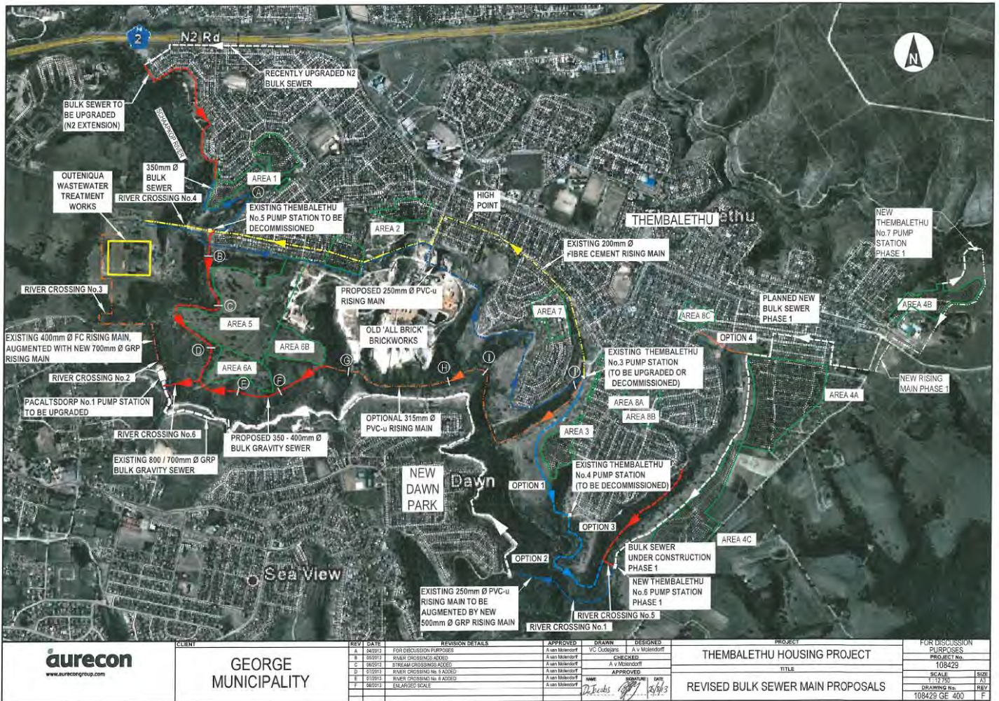
Figure 1. Layout of the Thembaletu UISP as provided by Aurecon, the project engineers. The bulk sewers and river crossings along the Schaapkop River are illustrated. Please note that the white and yellow lines on the above diagram indicate the existing sewer lines (not part of this
