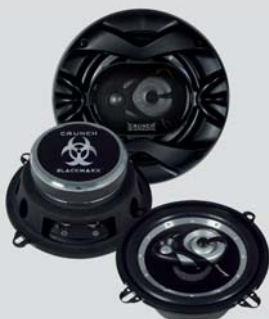
BMX53 5.25" (13 cm) 3-Way Triax-System 75/150 Watt, Impedance 4 Ohm ↓ 54 mm, Ø 115 mm
