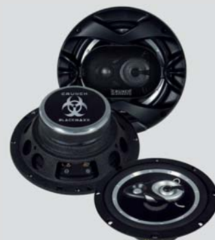
BMX63 6.5" (16,5 cm) 3-Way Triax-System 90/180 Watt, Impedance 4 Ohm ↓ 57 mm, Ø 145 mm
