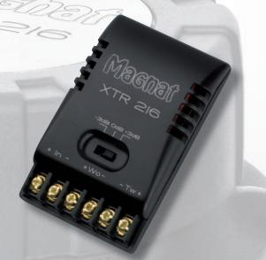
Very well-equipped crossover with 12 dB filters and even a trap circuit for the frequency response correction of the 16 cm system is present.
