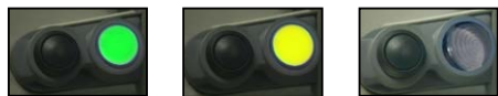
Dome lamps are on Liftgate battery is charging (16-7812TC only) Normal conditions/ Trailer dome lamps are off
