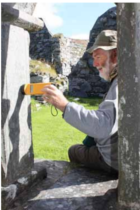
Figure 1: A KT-9 Kappameter NAR at use on the Isle of Oronsay 2013. Copyright David Caldwell
