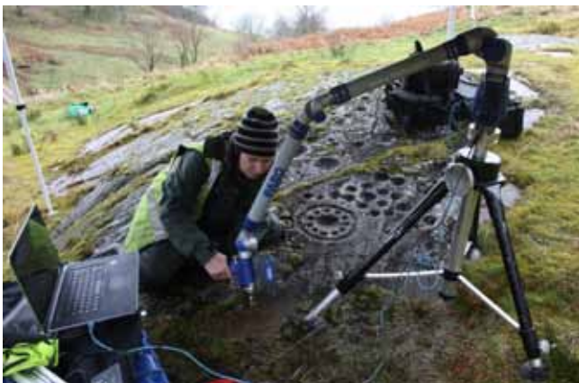
Figure 1: Recording Exposure 1 South using a Faro Platinum Arm with laser line probe under a protective canopy. High resolution sub-millimetre terrestrial laser scanning systems are typically susceptible to variable exposure conditions, with strong lighting a particular problem; during the 2014 survey a lightweight tent was used to provide shade for the scanning operations. Copyright Forestry Commission Scotland by AOC Archaeology
