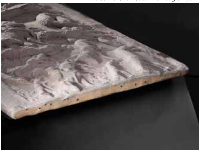
Figure 2: A cross-section through the 1849 plaster cast of the St Andrews Sarcophagus in the NMS shows how the craftsman reinforced it with iron rods. The cast was presumably cut up because the NMS, as it then was, wanted to correct Mr Ross's cast, which had reversed the arrangement of the monument's corner slabs. © Doug Simpson
