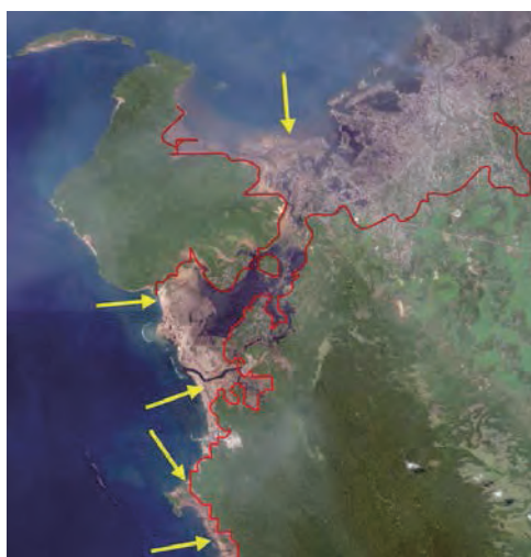
Fig. 24. The red line indicates tsunami inundation boundary in northwest Aceh Province, while the yellow arrows show directions of tsunami waves.
