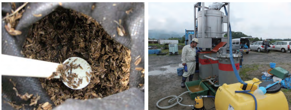
Fig. 4. Rice chaff (concentration of more than 30,000 Bq/kg radioactivity) after the test of decontamination of radioactive cesium (left), and a contaminated water purification system using rice-chaff named SEMJ-system (right).
