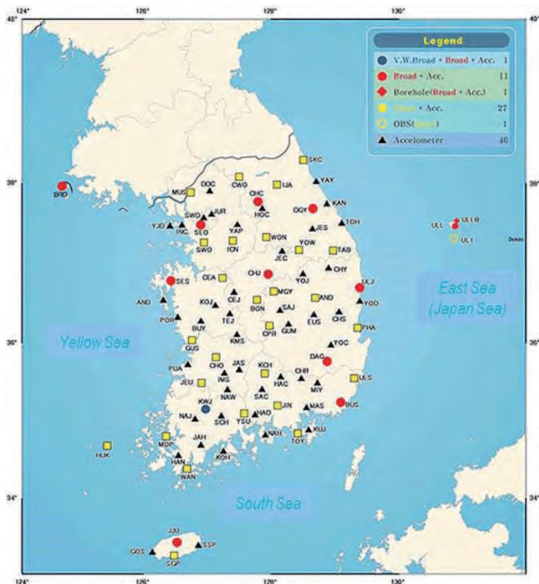
Fig. 6. The earthquake and earthquake-generated tsunami monitoring network in Korea which is jointly operated by KMA and KIGAM in Korea (KMA, 2013b). Both agencies are jointly monitoring natural or artificial movements of the earth crust, which are announced by KMA.
