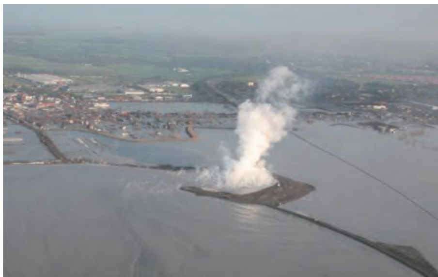
Fig. 2. Dikes constructed to control mud flow of Lusi, looking to the south. Steam dominates the mud volcano, rising as high as 100–150 m from the main crater which is extruding mud, water, gases, and a mixture rock fragments.
