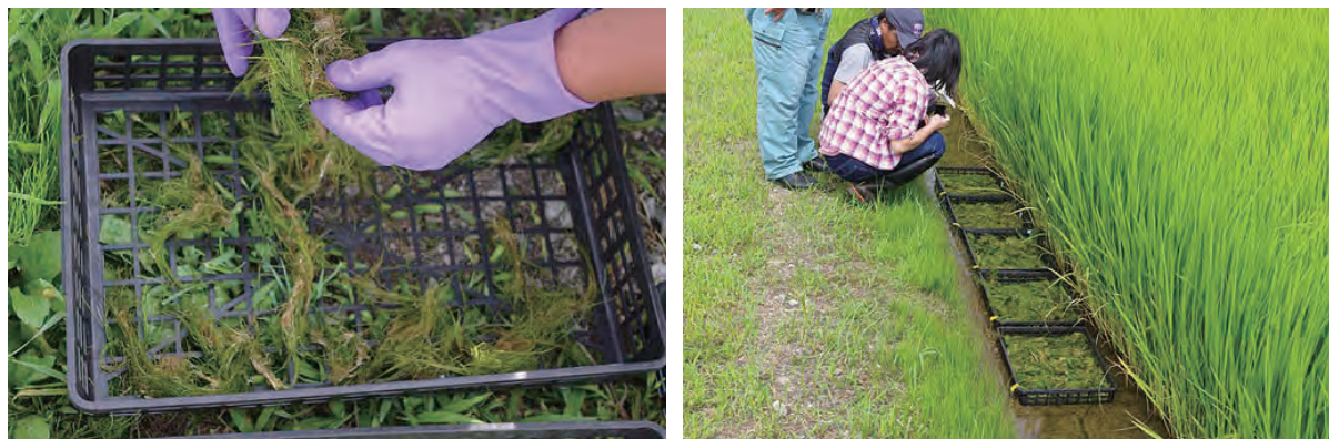
Fig. 3. Testing applicability of phytoextraction by Eleocharis acicularis of soil contaminated with ^{137}\text{Cs} in paddy field, Fukushima Prefecture
