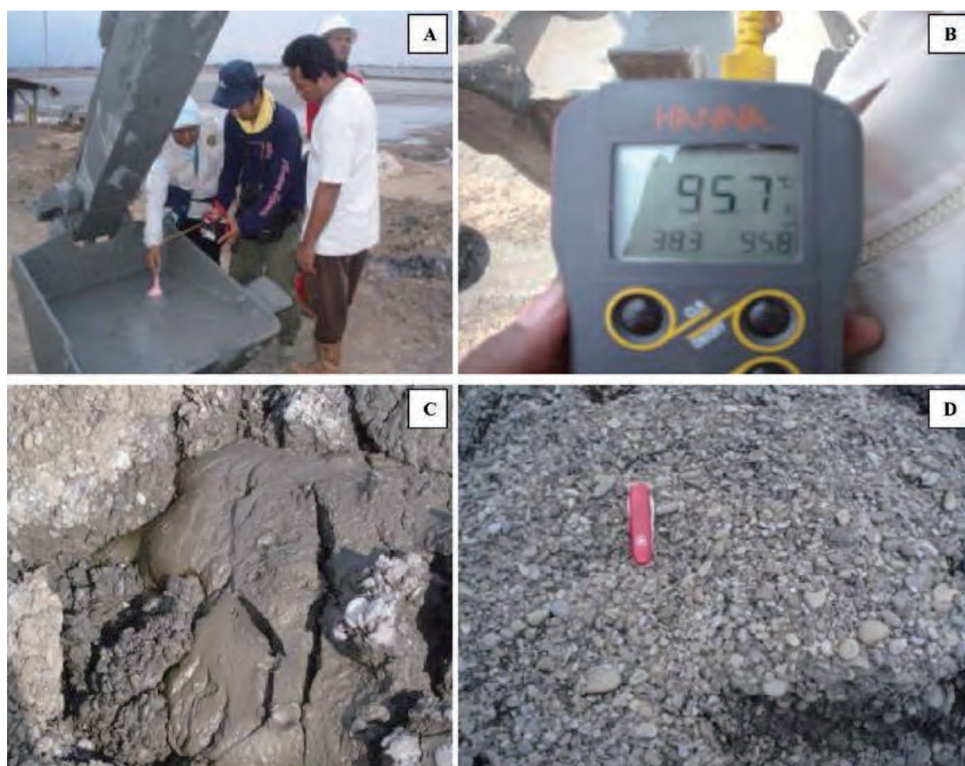
Fig. 3. Mud of Lusi composed mostly of water with fragments of shale, silt, andesite, tuff, and various minerals. The temperature of the mud is nearly at boiling temperature. A: Sampling hot mud of Lusi from the crater. B: Temperature (°C) of hot mud. C: Dried mud. D: Mud washed by rain.
