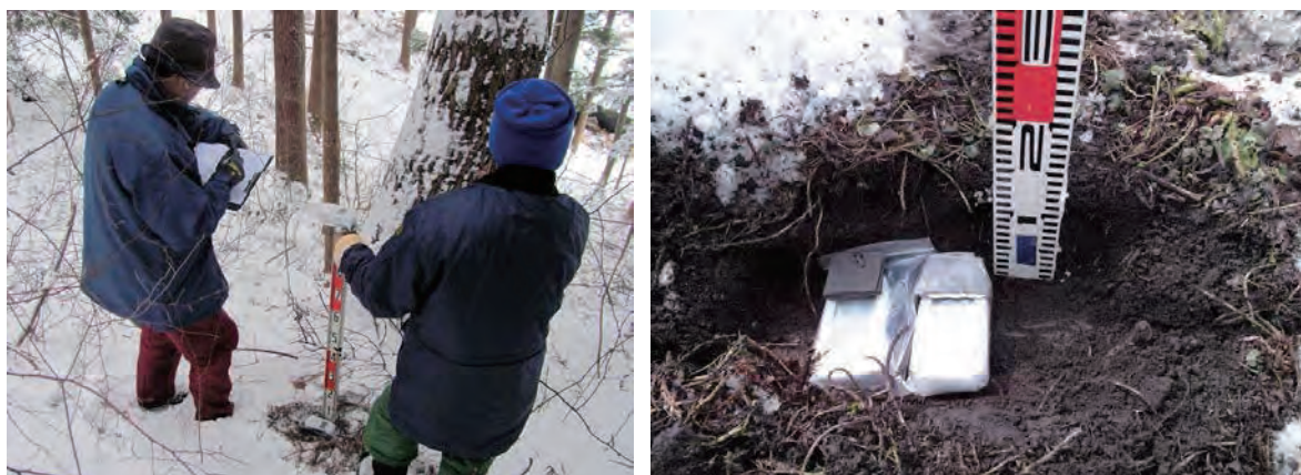
Fig. 5. Radiation dose measurements (left) from ground surface to 1.0 m height, and (right) at several depths below the ground surface, in which the radiation detector was capped by a lead box to shield from air radiation.
