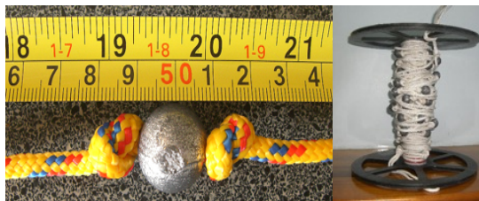
Figure 4. Left: close-up of transect line with lead weights (every 50 cm); Right: rolled up transect line.
