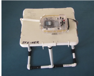
Figure 5. Quatripod with an image capturing area of 40 x 30.
