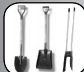
Post Hole Digger - hand held and Shovels - spade type and regular
