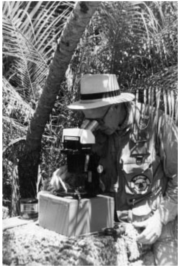
Fig. 8.5. A mirror used to focus sunlight on a specimen serves as a portable microscope lamp for examining scale insects in the field.
