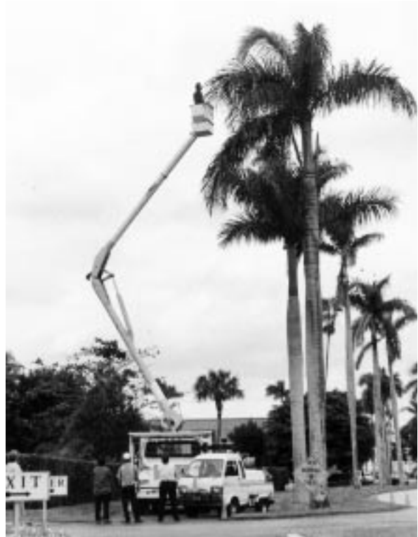
Fig. 8.2. A truck-mounted hydraulic-lift 'bucket' used in tree maintenance is useful for studies of palm insects. In Florida, city parks and streets departments have assisted research entomologists by making this type of equipment available to them.
