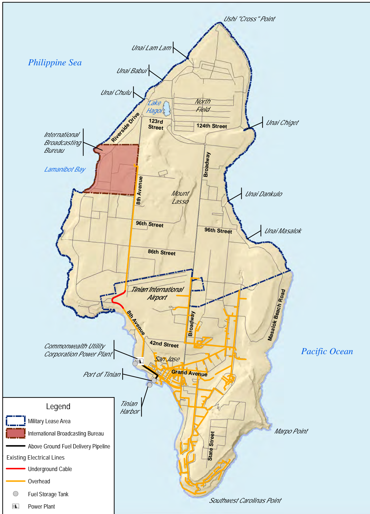
Figure 3.14-1 Tinian Power Distribution
