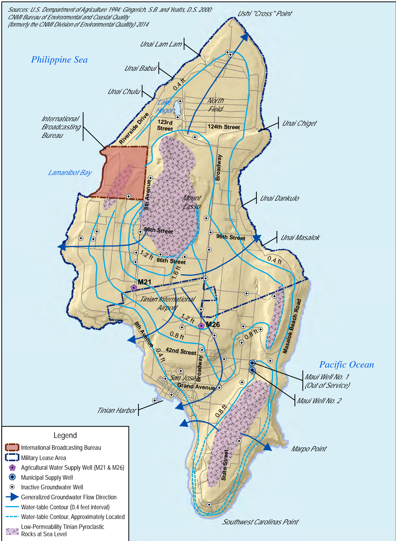
Figure 3.3-4 Tinian Groundwater Wells, Elevation, and Flow Direction
