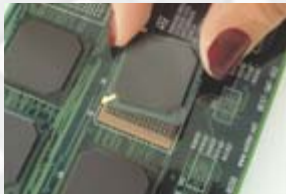
Step 4 - Align, place part and reflow
