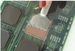
Step 3 - Squeegee paste or flux through the apertures onto the PCB
