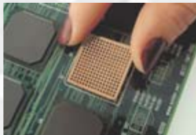
Step 2 - Align and affix the StencilQuik ™ onto the PCB
