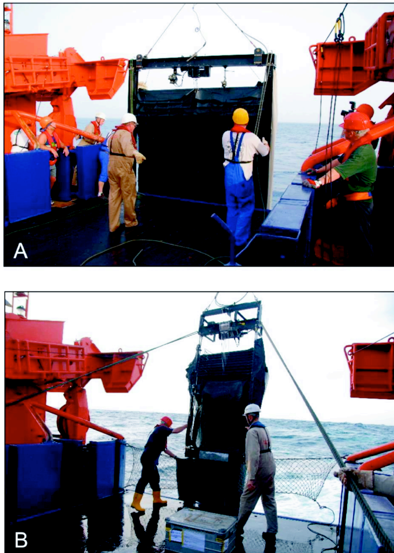
Fig. 3.1.1: Deployment of the 10-m 2 (A) and 1-m 2 (B) MOCNESS from the stern of the Polarstern. Note the net bar and deflector flaps on the MOC10 to prevent contamination of the samples from great depths with animals living at shallower depths.
