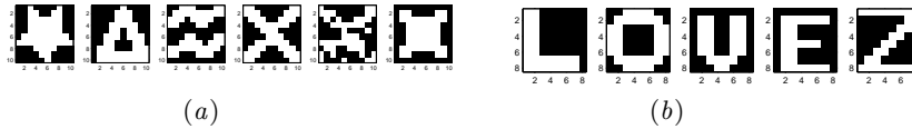
Fig. 5. The patterns used by Adachi et al (a) and Inoue et al (b). The first four patterns in (a) and (b) are used to train the network. The fifth pattern in (a) is obtained from the fourth pattern by including 15% noise. The sixth pattern in (a) and the fifth pattern in (b) are the untrained patterns.
