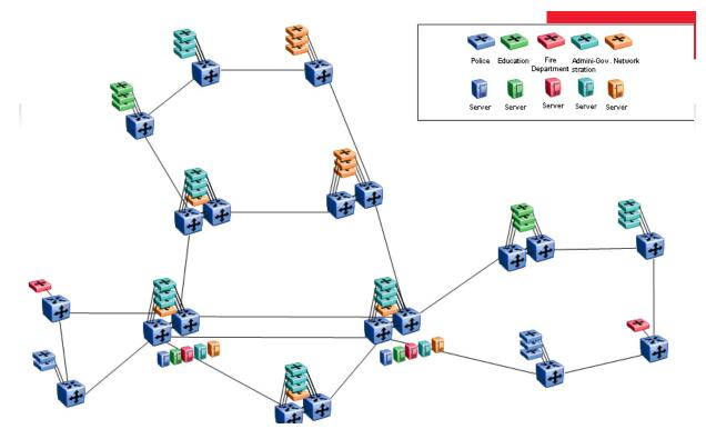
Figure 22 - Dual Homing of Access Switches into SPB Nodes
