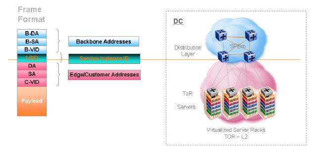
Figure 2 - 802.1ah Frame Format
