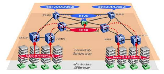
Figure 14 - SPB Inter-I-SID Routing
