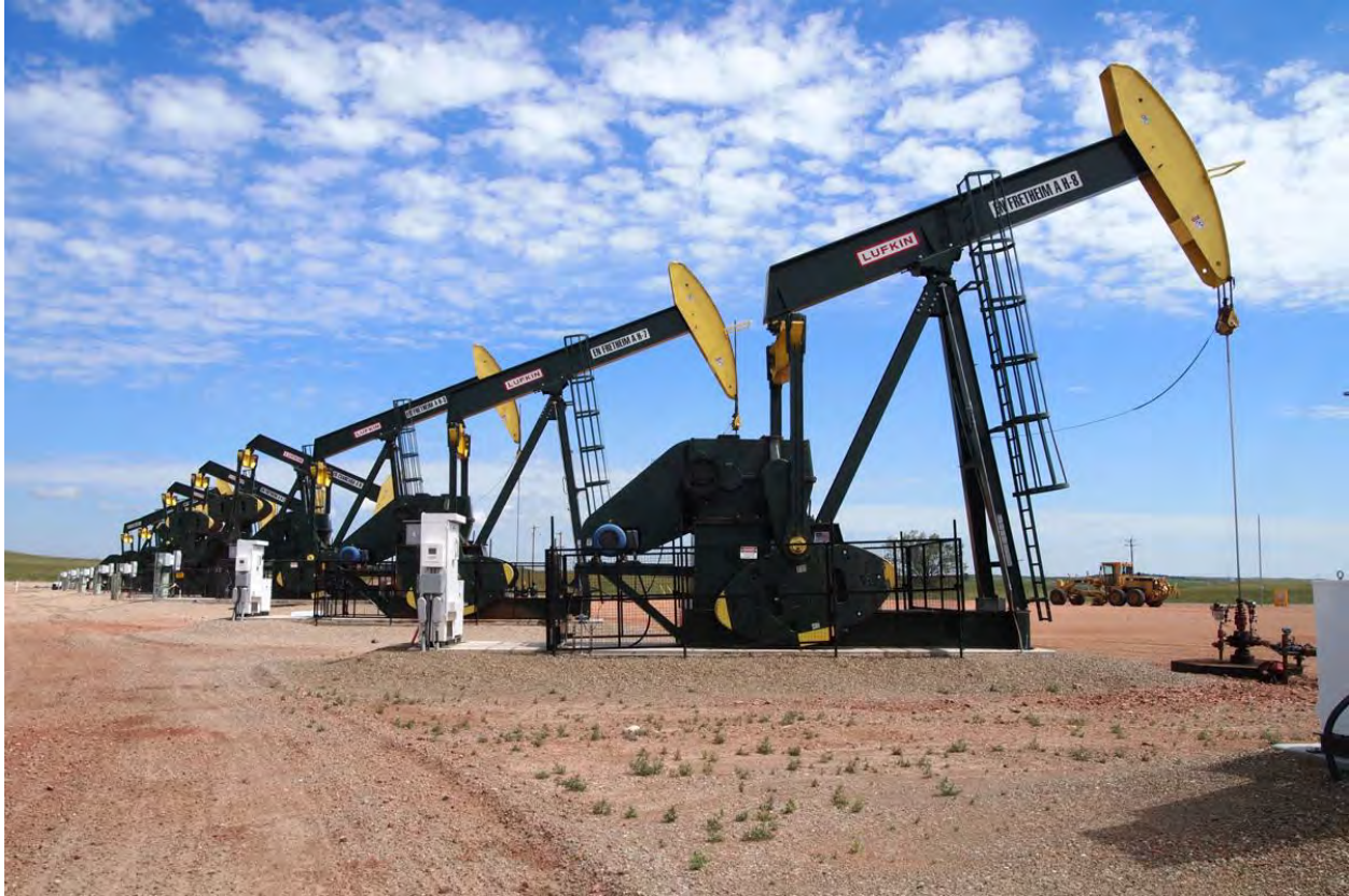
Pumpjacks in Mountrail County (Source: Bismarck Tribune)
