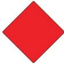
END OF ROAD
