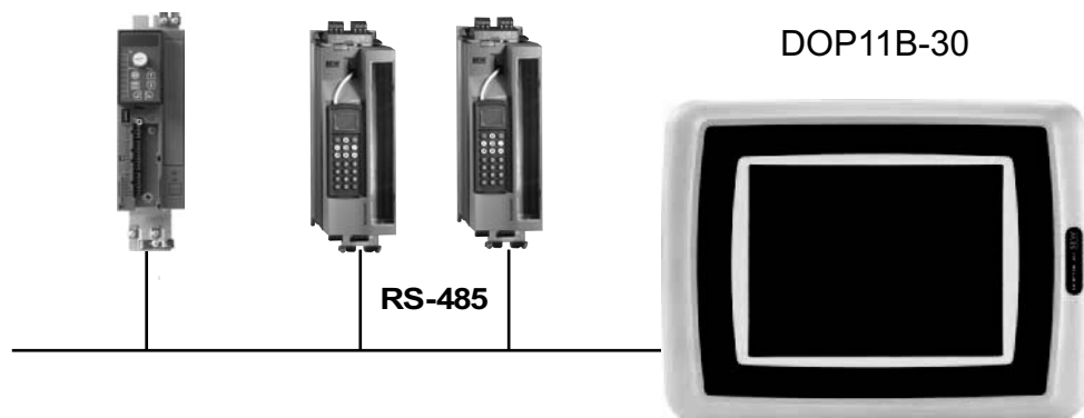
Figure 12: Connection between operator terminal and MOVIDRIVE® MDX60B/61B
