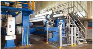
靴式压榨 Integra®-Shoe 可控中高压光机 Integra®-Calender
