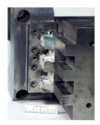
Figure 3. Typical Fuel Shear Blade Design (Croff, 1997).
