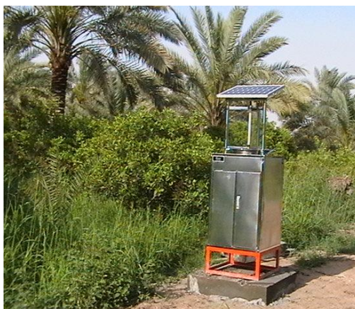
Figure 23. Solar light trap (Magna Trap with lamp of 320-420 nm wavelength, Russell IPM Limited, UK) used for monitoring and controlling Oryctes spp. in date palm orchards in Iraq (Photo: Mohammed Z. Khalaf)
