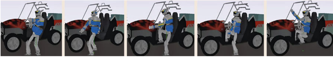
Fig. 67.42 Snapshots from multicontact planning and control of HRP-2 ingress in a car (after [67.121]). From the initial posture, supported on the steering handle and the seat by an arm, the robot finally succeeds in entering the car
