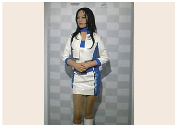
Fig. 67.5 Actroid (courtesy Kokoro), an android designed for entertainment, telepresence, and media roles
