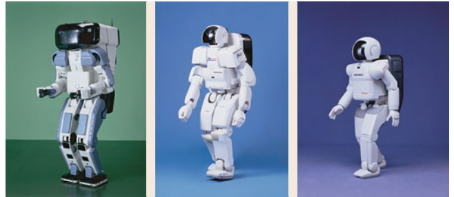
Fig. 67.9 (a) Honda P2 (180 cm tall, 210 kg), (b) P3 (160 cm, 130 kg), and (c) advanced step in innovative mobility (glossnoidx-ASIMO advanced step in innovative mobility) (120 cm, 43 kg) (after [67.31]; courtesy Honda)
