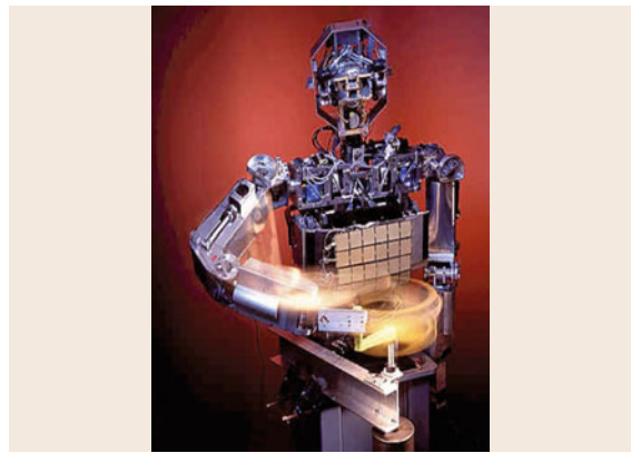
Fig. 67.10 The humanoid robot Cog used neural oscillators in conjunction with compliant torque-controlled arms to perform a variety of everyday tasks with human tools, such as crank turning, hammering, sawing, and playing a snare drum (after [67.32]; courtesy Sam Ogden)
