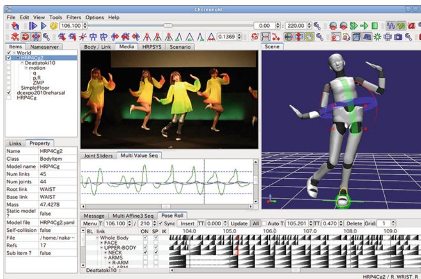
Fig. 67.28 A motion choreography tool working within the Choreonoid framework. In this tool, whole body motions of biped humanoid robots can be created with key-frame editing similar to computer graphics (CG) character animations (after [67.78])
