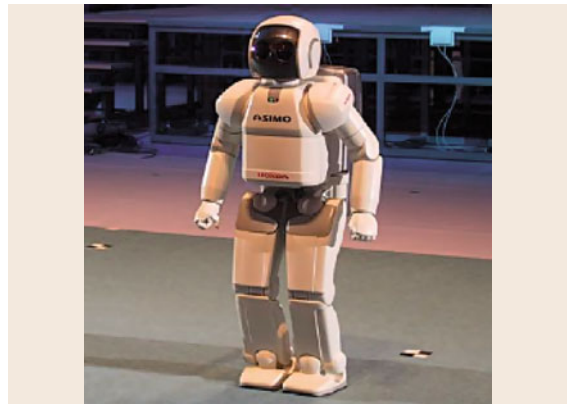
Fig. 67.22 ASIMO and artificial landmarks on the floor
