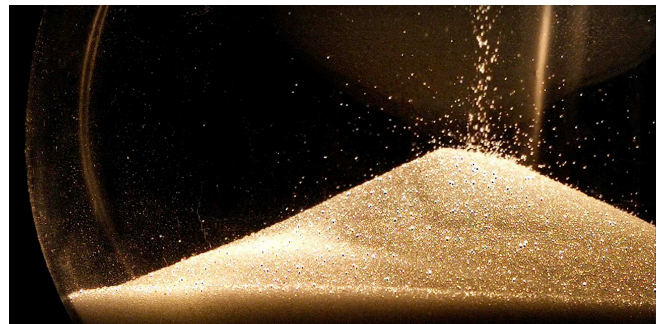
Fig. 10. Hourglass experiment: Individual grains bounce off a sand pile, violating the continuum assumption and requiring a discrete model. ©MIT
