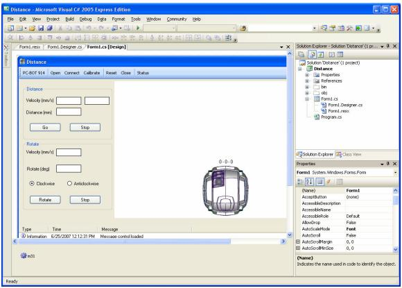
Sometimes the Form tabs do not open automatically when the project is opened. Click on 'Solution Explorer' in the top right part of the window and right click and open any of the Form1.cs and listed files to open them.
