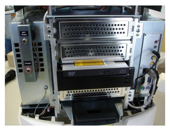
Plug the monitor, keyboard and mouse into the Mini-ITX back panel in order to setup your robot, like the network etc.
