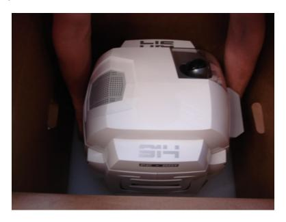
The following image shows where the handles are located, you'll have to feel for them when the robot is in the box. There are two handles front and back.
