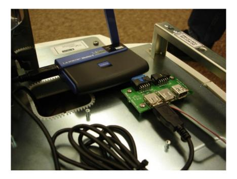
In this location the head can still be placed back on the robot and not interfere with the Wireless USB Network Adapter or its antennae.
