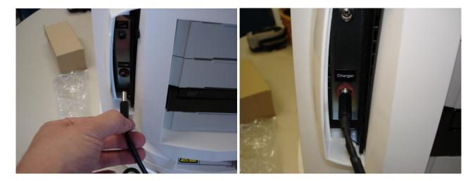
The charger LED will first be GREEN after the AC cord is plugged into the wall. It will then change to ORANGE when it is charging the batteries on the PC-BOT. It will then switch back to GREEN when the batteries are fully charged (it typically takes 2 -2.5 hours to charge the batteries from the auto-shutoff point).
