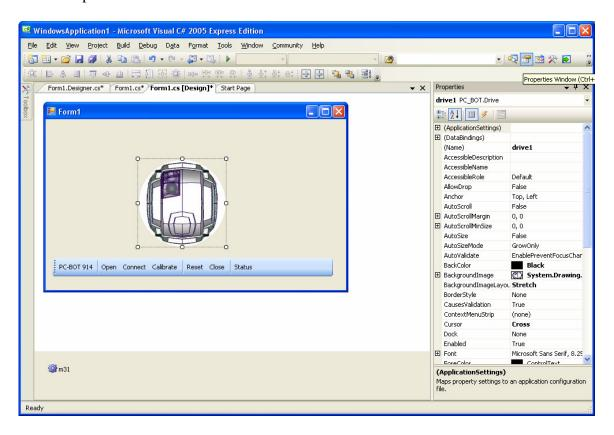
On **EACH** of the components you put in the Form1 windows, you need to connect them to the M3 component. In the 'Properties Window' scroll down until you see "**PC-BOTm3**". By default it is set to (none).
