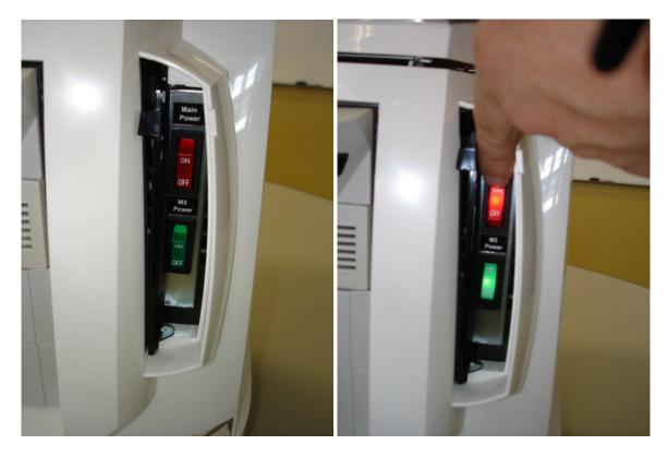
Switch on the Main Power switch (RED) **AND** M3 Power switch (GREEN) on the front of the robot. **WAIT 5 seconds** and the M2-ATX Power Supply will cycle the power to the PC automatically.
