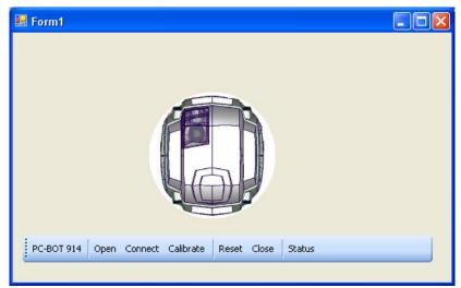
Same as with the sample applications included with the PC-BOT .NET components installed, you will need to first click on 'Open' then 'Connect' before trying to drive your robot motors by clicking and dragging the PC-BOT image.
