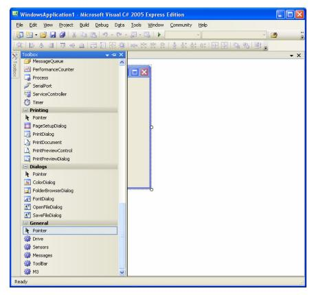
Drag and drop any of the PC-BOT components to the Windows Application Form screen and see what happens. For this example application the 'Drive', 'Toolbar' and 'M3' components were put in the Form.
