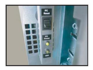
On the other side of the front of the robot, you can still use the PC ON and PC Reset switch just like on a regular computer.
