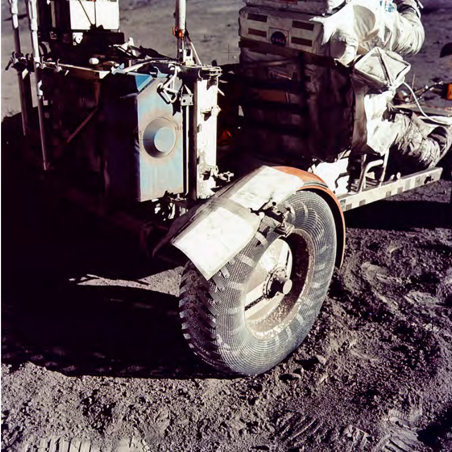
FIGURE 4. Rear wheel fender jury-rigged on the moon by astronauts of Apollo 17 from a plastic notebook parts, maps, and duct tape to prevent the abrasive lunar dust from hitting them while they drove and from damaging the rover.
