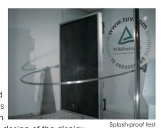
taken into account in the design of the display enclosure, for example, the connector protection covers can be attached to the rear panel of the display to help prevent water from leaking into the connectors situated on the rear panel.
