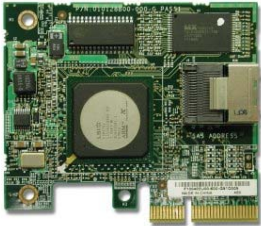
Figure 17. ServeRAID-BR10il SAS/SATA Controller v2 (BR10il v2)
