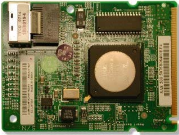
Figure 16. IBM ServeRAID-BR10il SAS/SATA PCIe Controller
