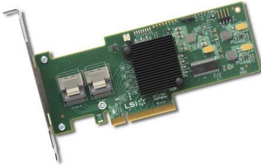
Figure 9. IBM 6Gb SSD Host Bus Adapter
