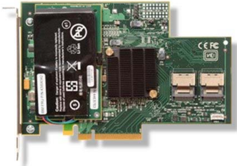
Figure 13. ServeRAID-MR10is VAULT SAS/SATA Controller
