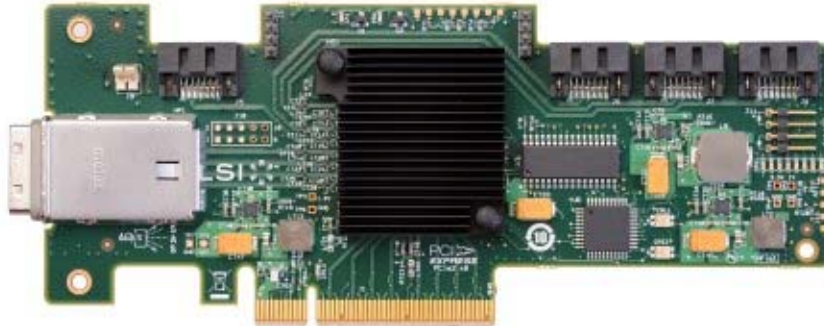
Figure 8. IBM 6Gb SAS Host Bus Adapter with the PCIe slot bracket removed
