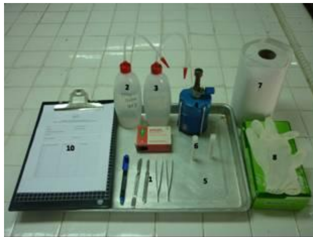
Figure 4: List of materials and tools for tissue collection
