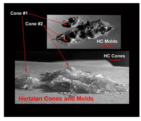
Figure 23 Hertzian cones, bottom, and the molds in overburden at top, seen upside down.
