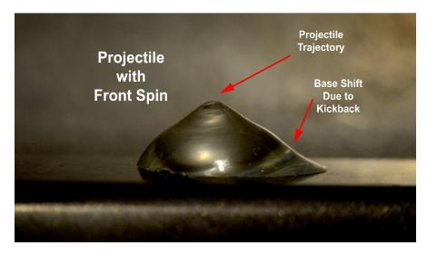
Figure 20 A Hertzian cone with base shifting due to a forward spinning projectile.
