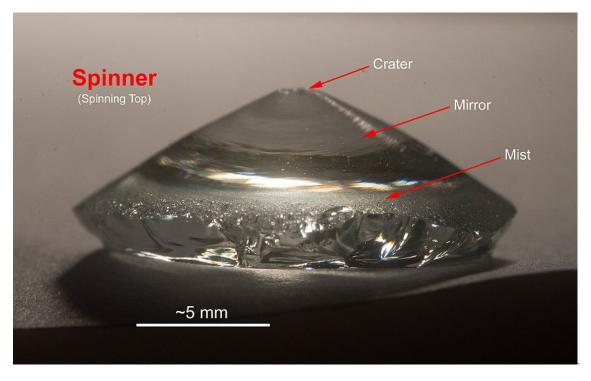
Figure 36 A spinning top (spinner) segment of a Hertzian Cone. Sizes vary with percentages of cone fragmentation.
