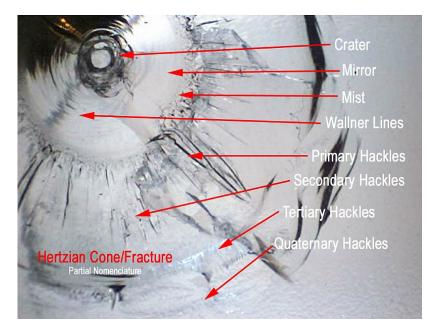
Figure 9 Sequential divisions in a compound Hertzian cone.
