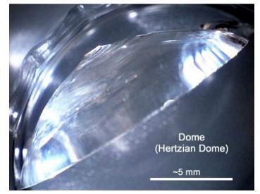
Figure 12 A simple domed HC with pedestal in profile.
