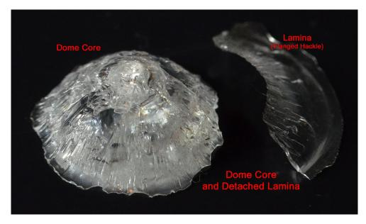
Figure 13 A domed HC core with detached flanged lamina.
