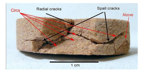
*Figure 42* T.J Ahrens, et al, Cal Tech. Image of spallation in Coconino sandstone. Note the circular features in the main spall and the alcove to right of image. Red lettering and arrows added for this glossary.
