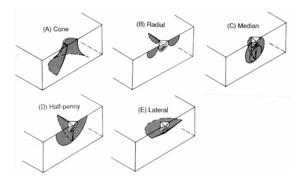
**Figure 39** Terms used in: A General Introduction To Fracture Mechanics and Mechanical Strength of Materials Or: Why do things break and what can we do about it? Figure 36, den Toonder, Jaap M.J., Unclassified Report, © Philips Electronics 1998
