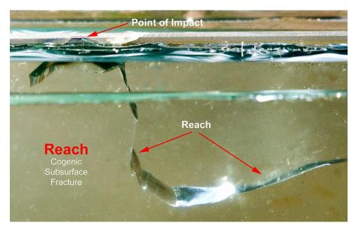
Figure 31 Subsurface fractures under impact HC's that "dive" into the target material.
