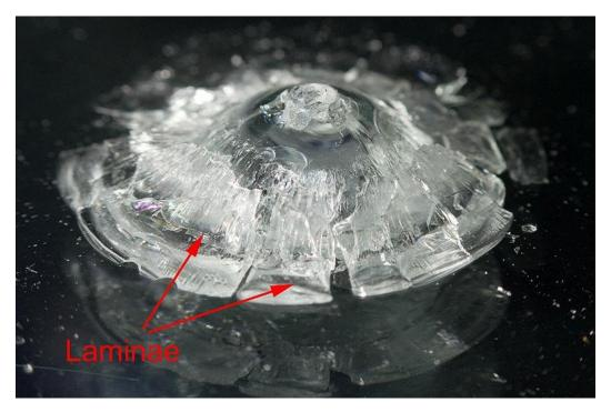
Figure 26 Detached laminae (flakes) with flanges. The Dome Core can be seen inside the outer band.
