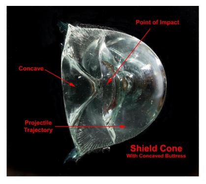
Figure 35 Shield Cones may occasionally have concave buttresses.
