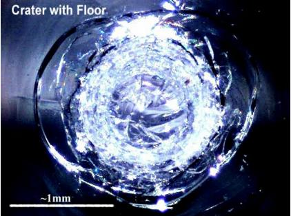
**Figure 19** A crater floor that remained in the crater as part of the overburden. Floor follow is the result when the cone was removed as in Figure 17.
