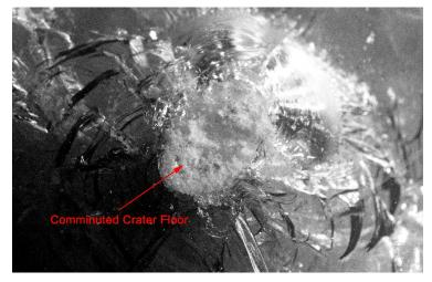
Figure 6 Comminuted, crushed material in a soda-lime glass crater.
