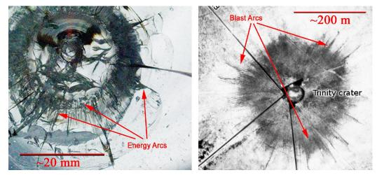
Figure 3 Energy dispersal patterns in HC, left, and nuclear blast, right.
