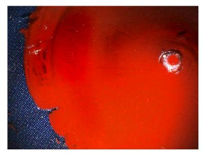
**Figure 1** Above, a stained Hertzian fracture mold exhibits (from left) flange and lobes, hackles (indistinct), terrace, crater and Wallner lines. All are within a radius of about 12mm.
