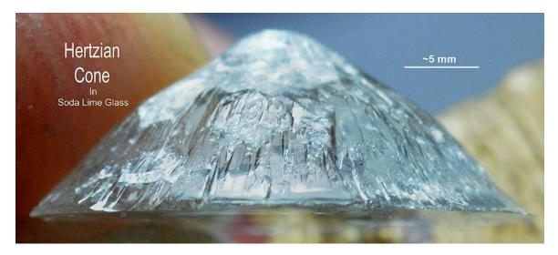
Figure 22 A 25mm diameter Hertzian cone replicates a mountain. The finger tip holding it can be seen in left background.
