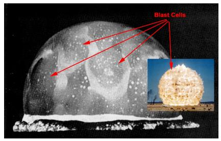
Figure 4 Blast cells in nuclear blast.
