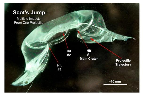
Figure 33 Scot's Jump. Illustrated is a sample of a three-hit, Hertzian fracture in soda lime glass created by a spinning projectile.
