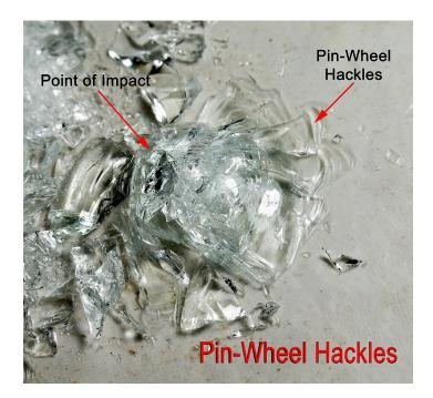
Figure 29 A highly fragmented Pin-Wheel shaped HC with large, lobed hackles.
