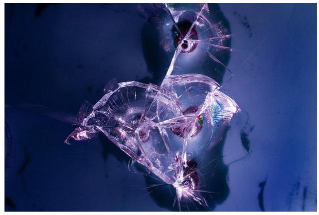
*Figure 24* Multiple hits in a sheet of soda lime glass from below. Cracks can indicate the sequence of impacts by studying the radial fractures. Later cracks generally do not cross the earlier fracture line.
