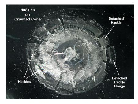
Figure 21 View of a segmented, crushed Hertzian cone. Laminae may divide radially, annularly and internally.
