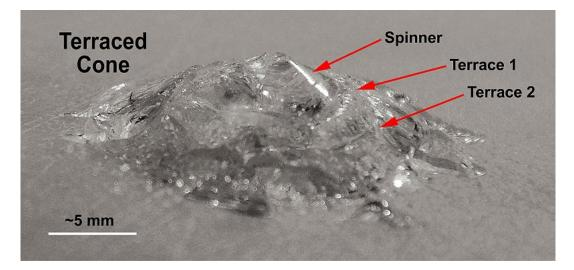
Figure 37 A Terraced Cone with two tiers and star-like radial lobes.
