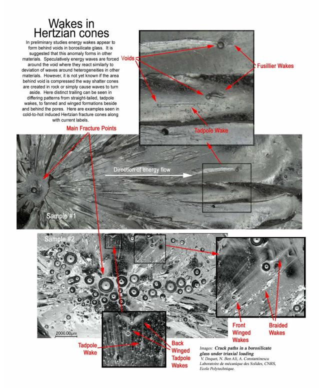
Figure 32 Wakes on the lee side of voids in borosilicate glass after fracture.
