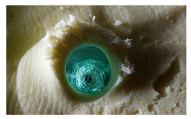
Figure 10 A crater and sub-surface Hertzian cone. A combination of 5mm soda lime glass and a "crustal" coating of modeling clay. The crater was made by a 5mm steel projectile.
