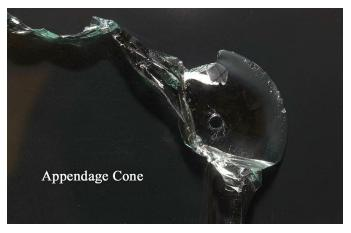
Figure 2 Appendage Cones are attached to overburden.
