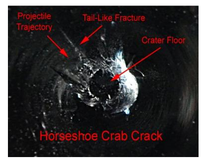
Figure 25 Horseshoe Crab Cracks can indicate the trajectory of the Projectile.
