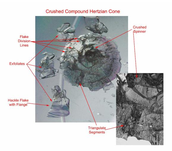
*Figure 7* A crushed compound Hertzian cone segments under polarized light. Triangulate segments are seen at right.
