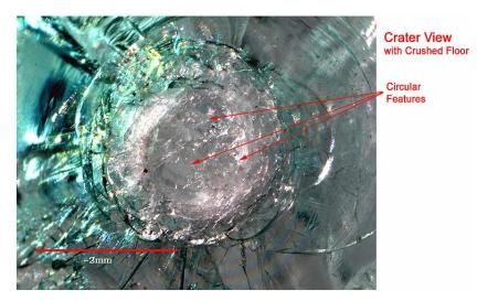
Figure 11 Crater in soda lime glass with CSA features (Compression Cells).
