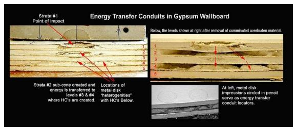
Figure 14 Energy conduits create sequential HC's through heterogeneities in gypsum board.
