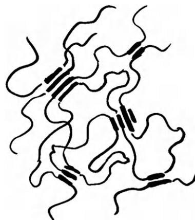
Figure 13.1 Schematic of the structure of a thermoplastic elastomer.
