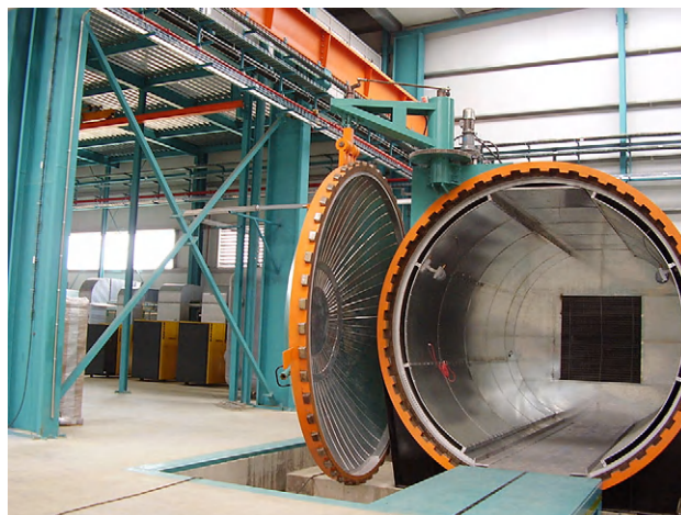
Figure 1.22 Picture of a large industrial size autoclave. For color version of this figure, the reader is referred to the online version of this book.
