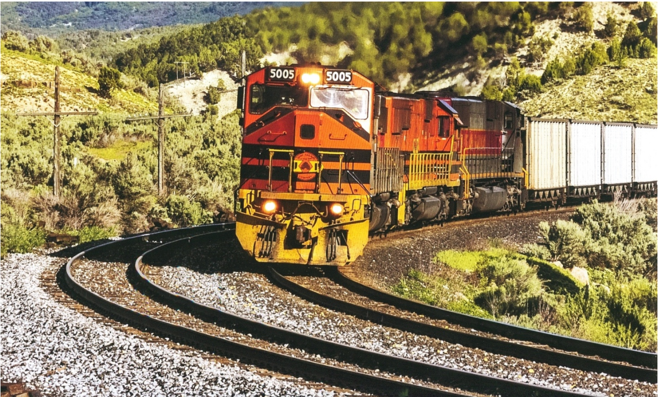
Curve on Heavy-Haul BSNF Rail Road in USA – No Check-Rails
