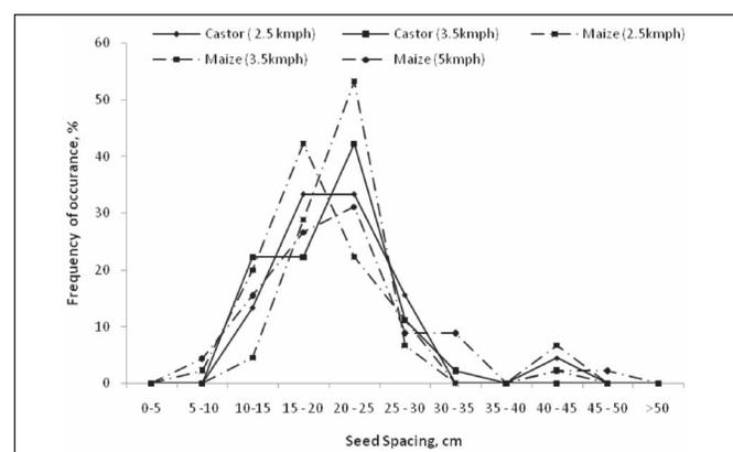
**Fig 5 : Seed spacing distribution pattern of incline plate metering mechanism**
