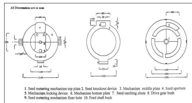
Fig 2 : Horizontal plate metering mechanism design details
