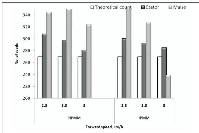
Fig 3 : Comparison of seed rotors in terms of number of seeds metered at different speeds
