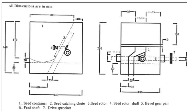
Fig 1 : Inclined plate metering mechanism with seed box
