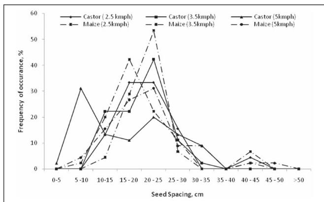
**Fig 4 : Seed spacing distribution pattern of horizontal plate metering mechanism**
