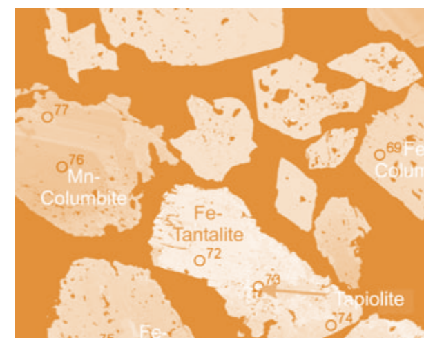
Figure 3: Back-scatter electron image of a columbite-tantalite concentrate from Rwanda displaying heterogeneous chemical composition shown by different grey values. Numbers refer to EPMA spots.
