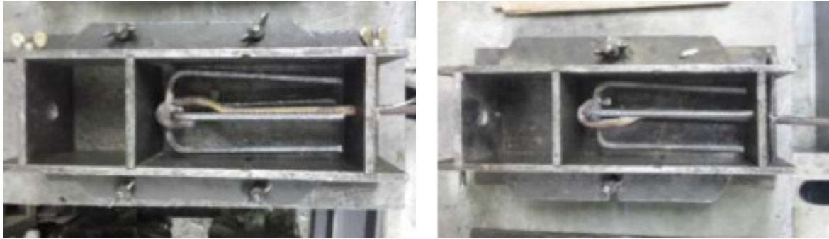
Fig. 4 Pattern (100 x100 x 300 mm) with corresponding partitions and anchorage for concrete
