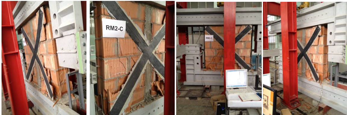
Fig. 5 Failure mode for RM2-C [6]
