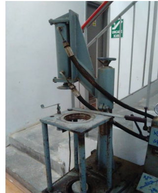
Fig. 2 Hydraulic compaction jack
