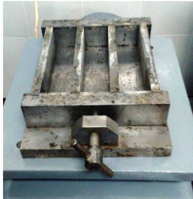
Fig. 1 Mould with three chambers
