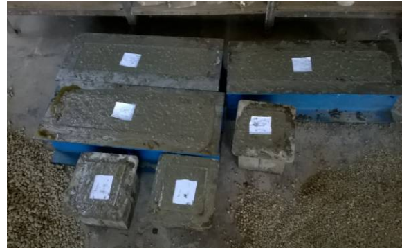
Fig. 2 Fresh concrete specimens
