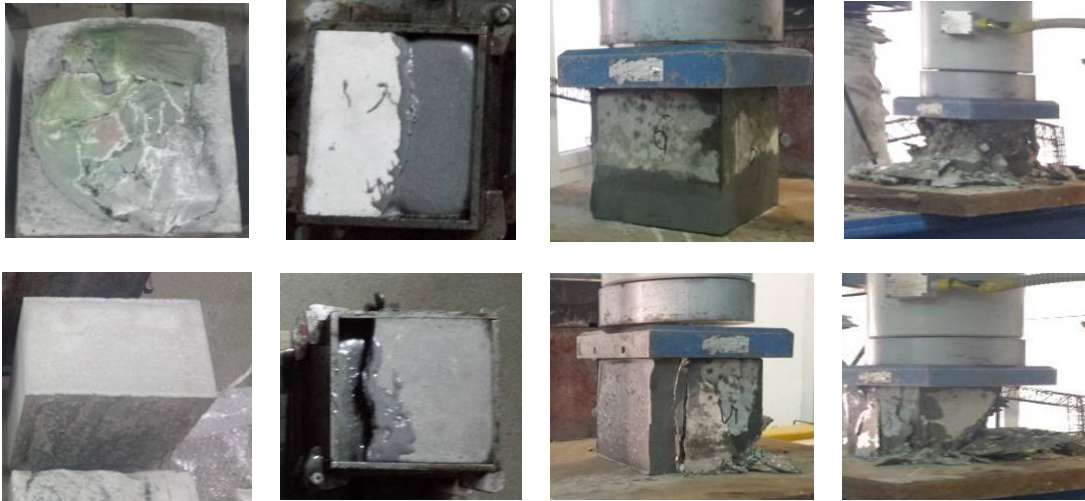
Fig. 2 Process of the testing: Concrete cube specimens / Addition of epoxy resin system / Compressive strength determination according to SR EN 12390-3
