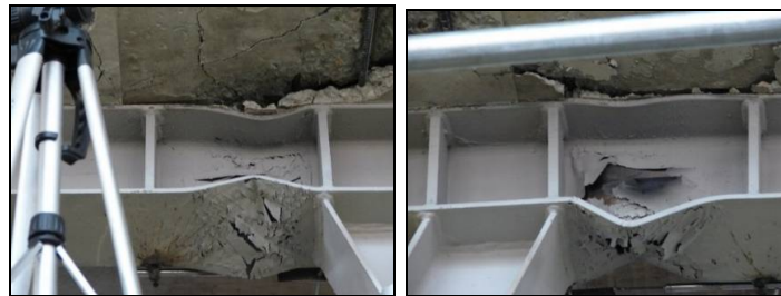
Fig. 5 Dissipative behaviour of the beam without connectors on dissipative zones – left and right side of the link
