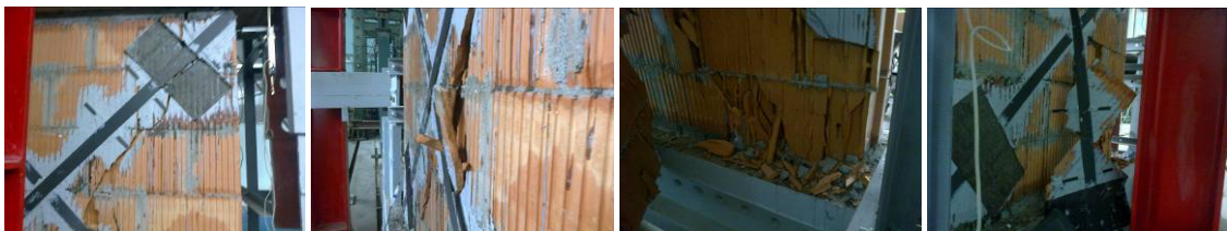
Fig. 3 Failure mode for URM1-C [6]
