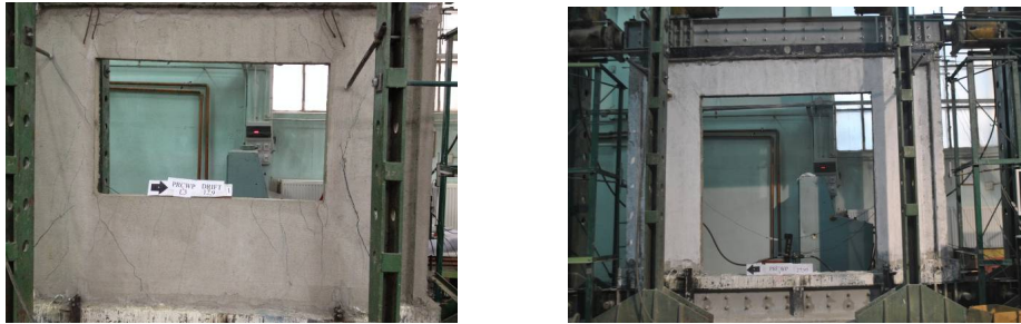
Fig. 2 Failure details of the specimens
