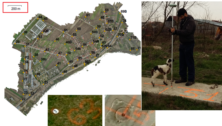
Fig. 1 Placing the Ground Control Points (GCP) on ground, materializing and determining their position
