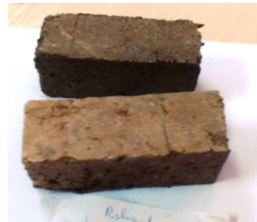
Fig. 5 Soil-cement testing sample
