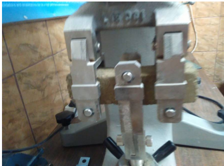
Fig. 4 Flexural tensile strength testing apparatus
