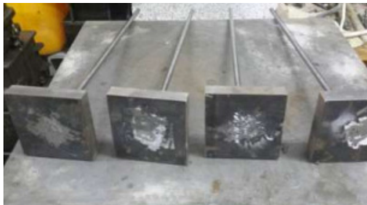
Fig. 5 Metal plates with anchors
