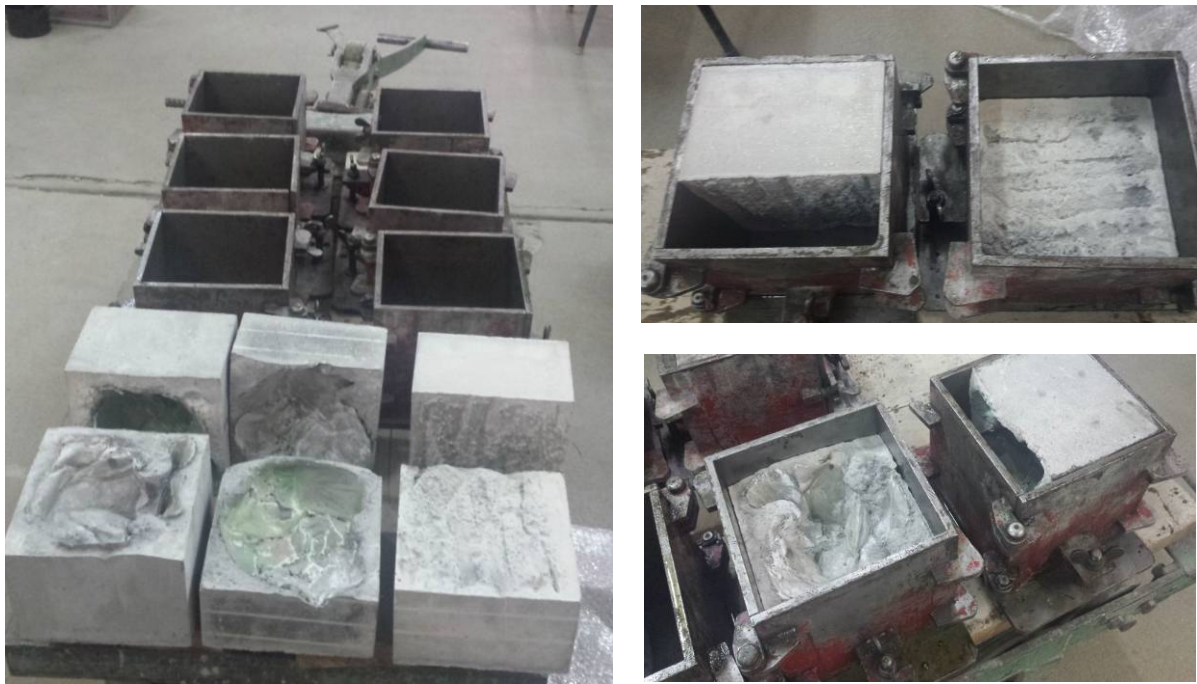
Fig. 1 Concrete cube specimens (150x150 mm) with cavities and furrows, prepared for testing
