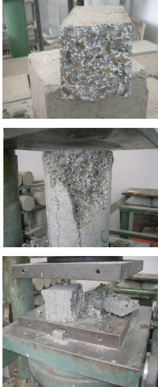
Fig. 1 Experimental tests on concrete with polystyrene granules
