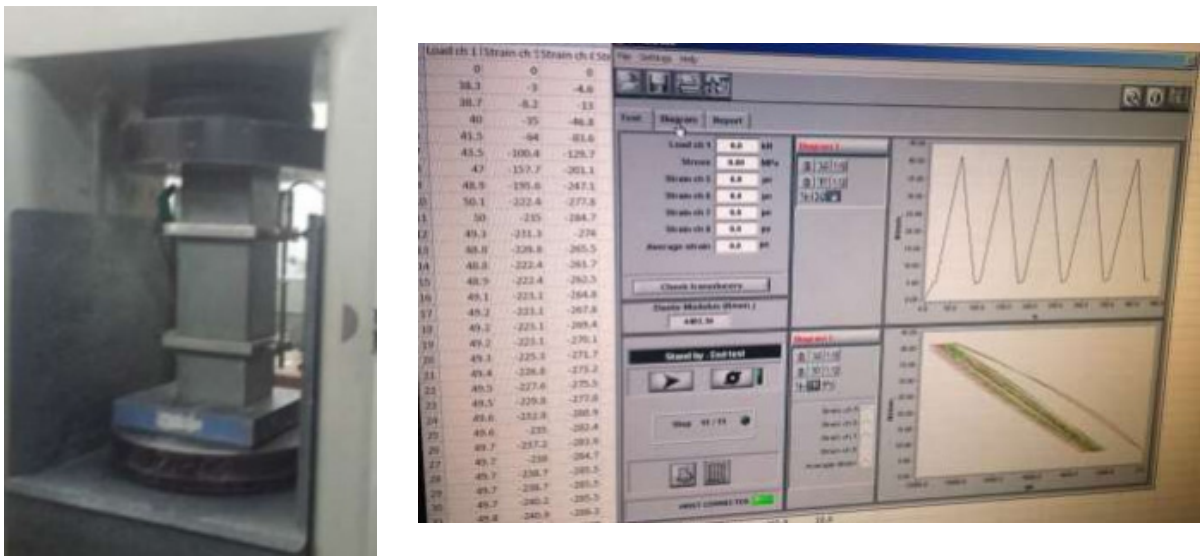
Fig. 3 Analyzing the module of elasticity of specimens (100 x100 x 300 mm) made of epoxy resin solvent
