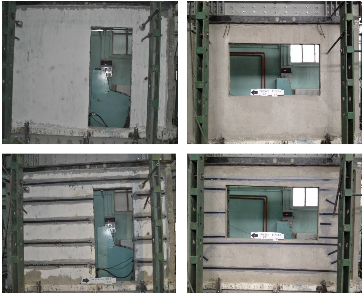
Fig. 1 Tested specimens, basic and retrofitted; left (PRCWP L1-E1), right (PRCWP L3)
