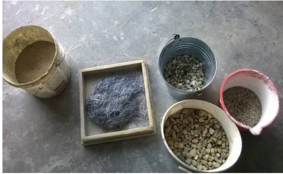
Fig. 1 Steel fibres and aggregates
