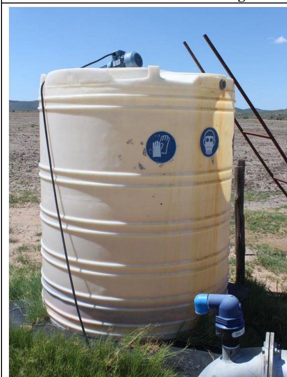
Photo 4-7 Fertiliser mixing tank
