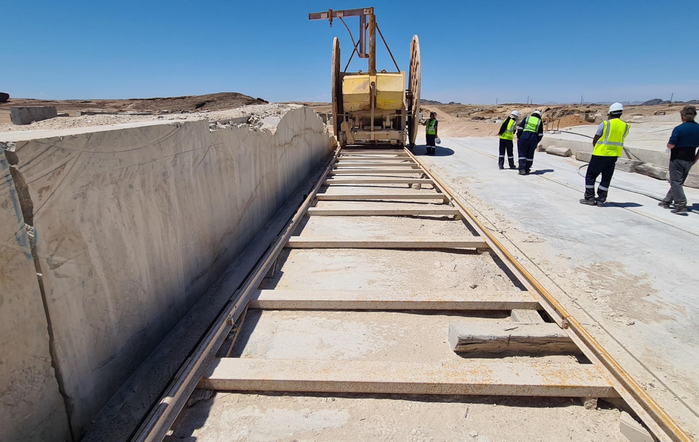
Plate 2.8: Giant saw used in the extraction of the granite blocks.
