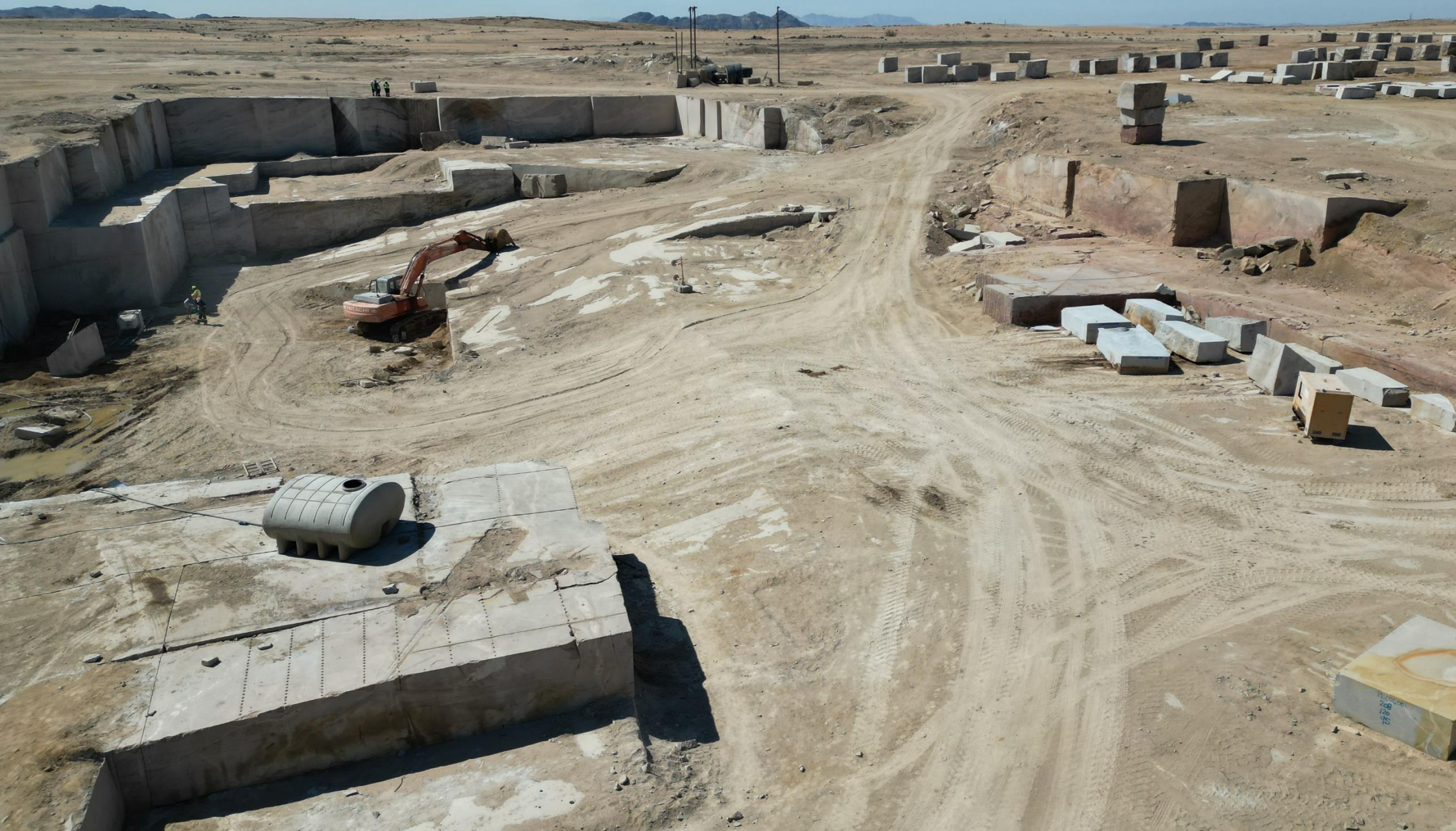
Plate 2.2: Drone image showing the eastern view of the working / extraction faces and floors and extracted small 2 m x 1 m x 0,6 m (majority), and larger blocks 2,8 m x 1,3 x 0,8 m (minority) rectangular blocks at a granite quarry in the ML No. 120.
