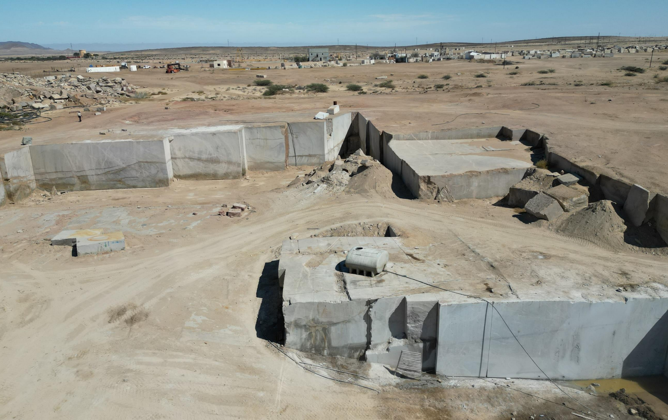
Plate 1.2: Detailed overview a granite quarry operational area, stockpile, sorted waste blocks for reuse and workshop and processing operations.
